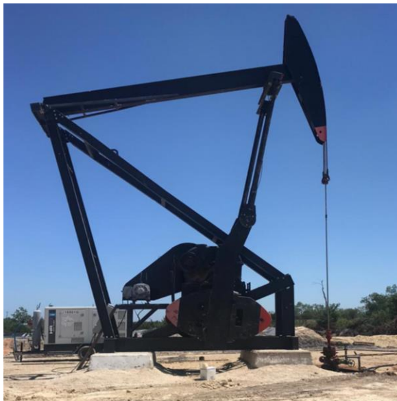
Figure 1: Beam pump producing oil at White Hat 2106
